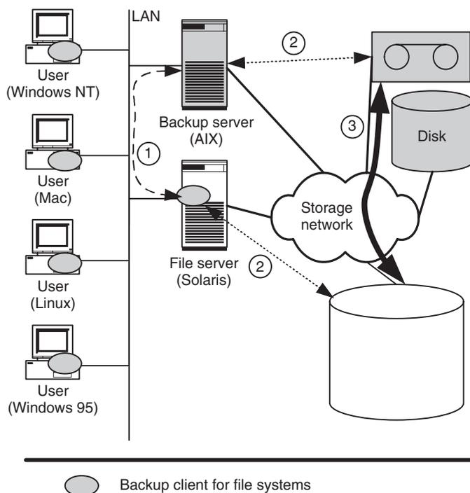
**Figure 7.7** In server-free backup, backup server and backup client exchange lightweight metadata via the LAN (1). After it has been determined which data blocks have to be backed up, the network backup system can configure the storage devices for the data transfer via the storage network (2). The heavyweight file contents are then copied directly from the source hard disk to the backup medium via the storage network (3).
