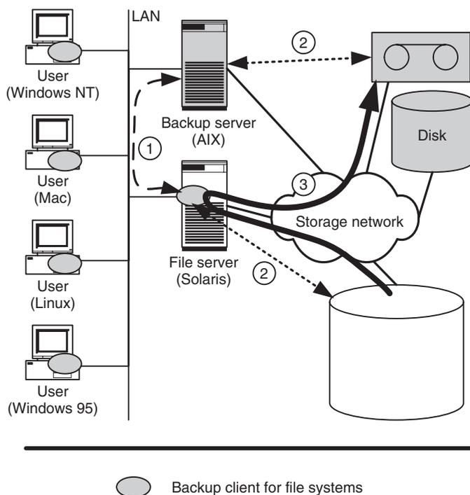
**Figure 7.8** In LAN-free backup too, backup servers and backup clients exchange lightweight metadata over the LAN (1). The backup server prepares its storage devices for the data transfer over the storage network and then hands control of the storage devices over to the backup client (2). This then copies heavyweight file contents directly to the backup medium via the storage network (3).
